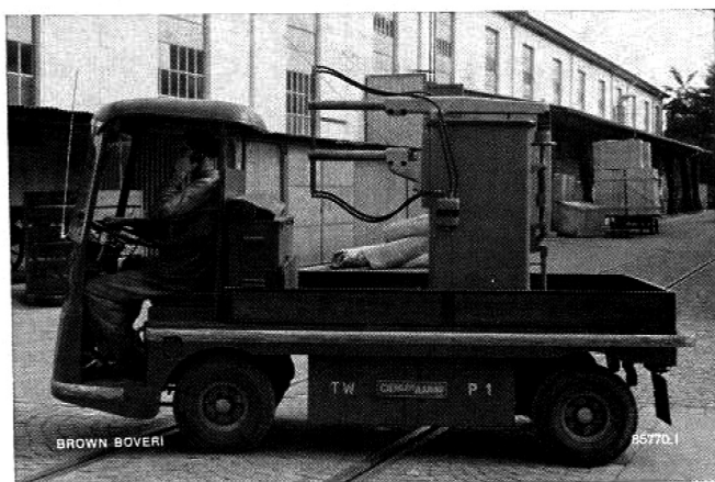
Fig. 7. — Internal factory transport is more economical when trucks, lorries, fork-trucks and cranes are directed by radio
