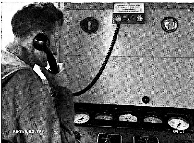
Fig. 6. — Shunting is accomplished more smoothly and with greater certainty using a radio-equipped locomotive
