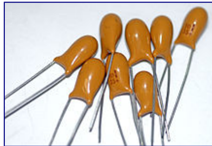
10 \mu F 30 VDC-rated tantalum capacitors, solid electrolyte epoxy-dipped style.
