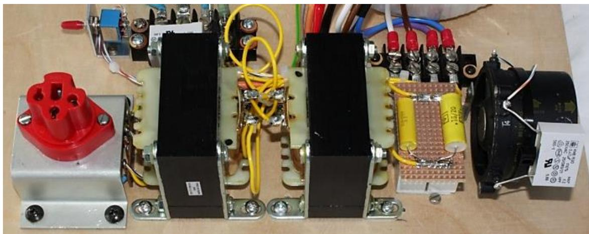
Figure 11. Layout of the output filter
