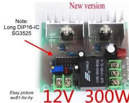
Figure 5. The Chinese inverter module
