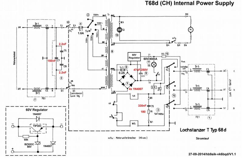
Corrosion on capacitors and solder lugs required a new strip, some rewiring and new capacitors. Silicon diodes replace the selenium rectifier. The resulting high voltage is regulated to 60V mainly to protect the end-of-line lamp (11).
