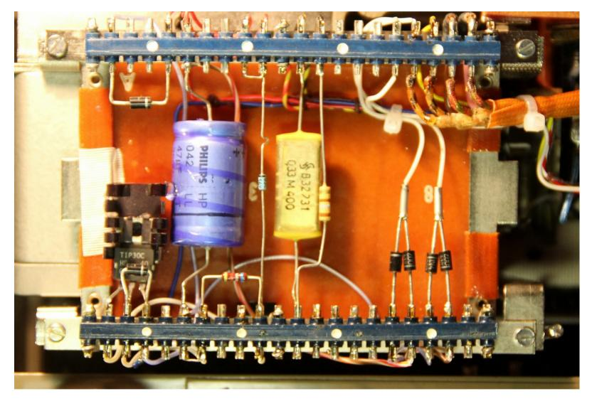
The power supply between the EMC filter and the bottom plate in this Swiss version provides line current for local punching operations (and the endof-line lamp). The machine was often used to prepare punched tapes for later transmission on other systems.
