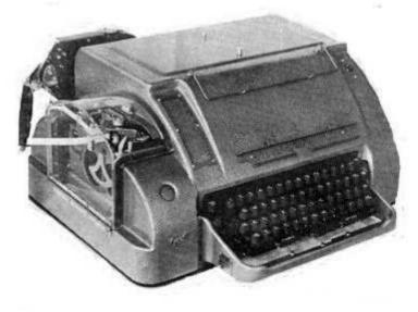
The component parts have many similarities with the model 7, from which it was developed. Like the model 7, a governed motor was normally fitted. This machine was allocated the Post Office reference number "Teleprinter No. 11".
