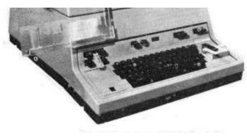
model 7 in the Telex and private wire services. It was designed to operate continuously at 75 Bauds, and was only provided with gears for 50 and 75 Bauds. It
