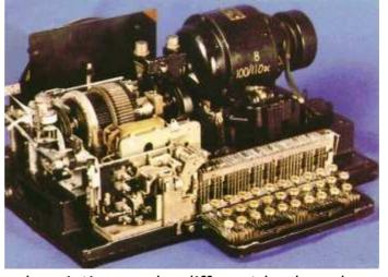
or B in place of the X in the description, and a different keyboard layout. It is possible to interwork between machines coded for Murray code and ITA2, provided that care is taken. A governed motor is fitted as standard, which may be adjusted to operate at 45.45 or 50 Bauds.
