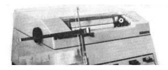
444 This page printing teleprinter was introduced in 1966 to replace the ageing
